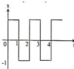
What is the (approximate) ratio of power in the 7th harmonic to the power in the 5th harmonic for the above waveform?
